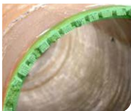
Core bit with teeth before welding tungsten carbide
