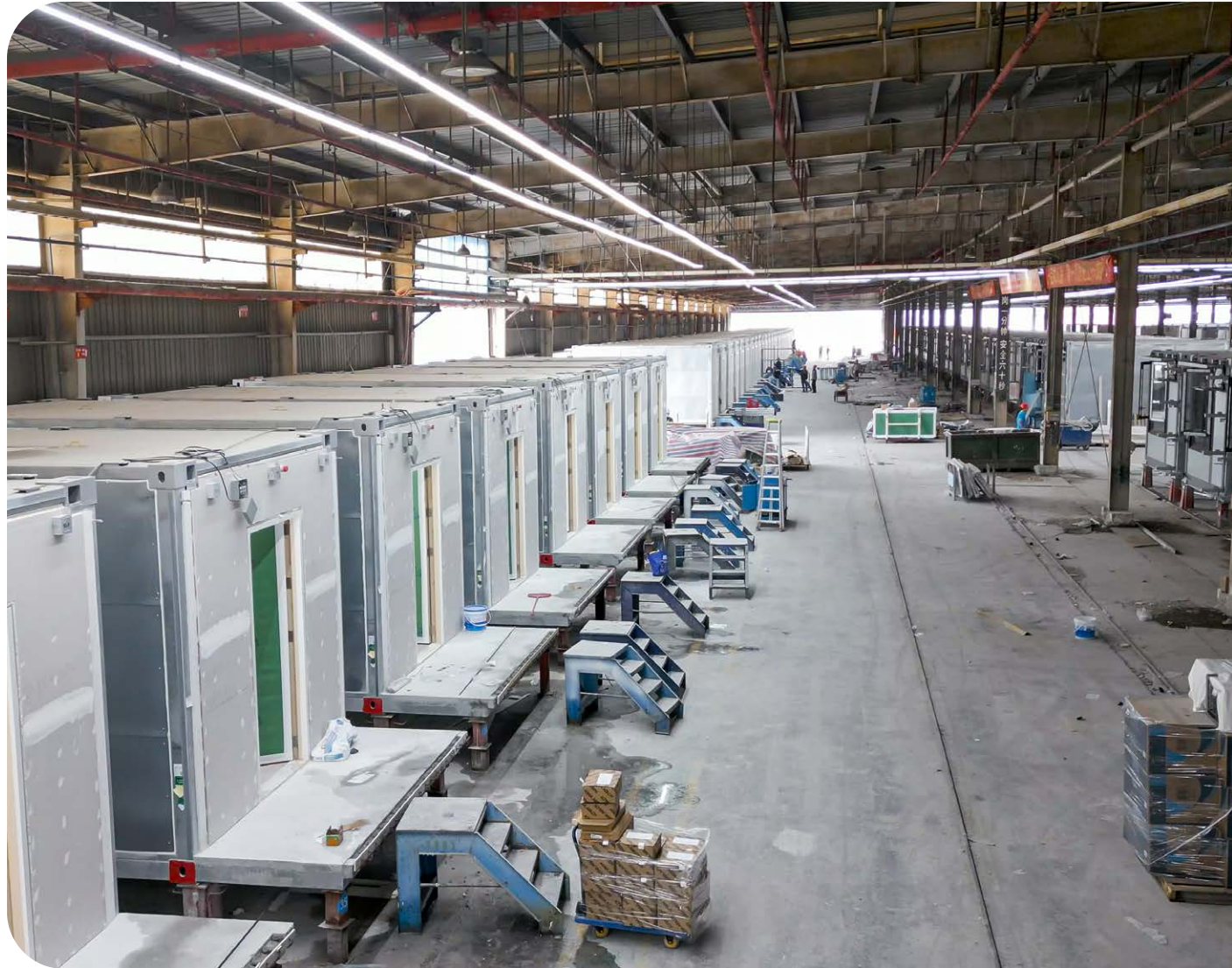
CityU student hostel units under construction at the factory
