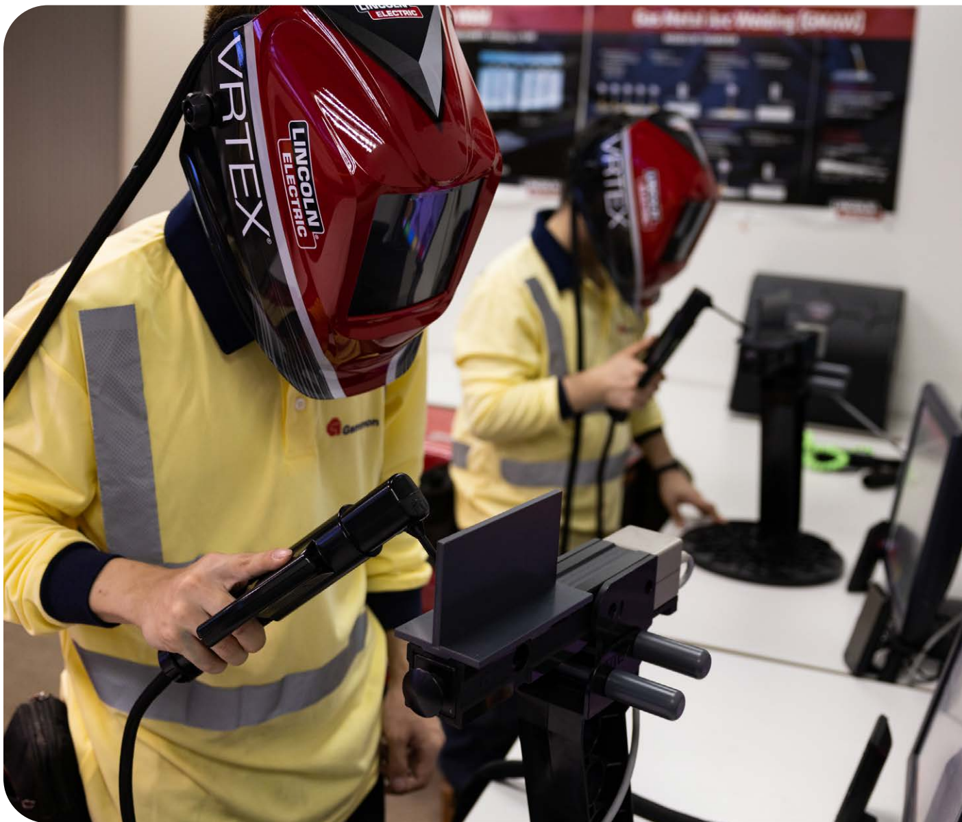
Staff hone their practical skills using a welding simulator
