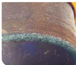
Core bit with teeth after welding tungsten carbide
